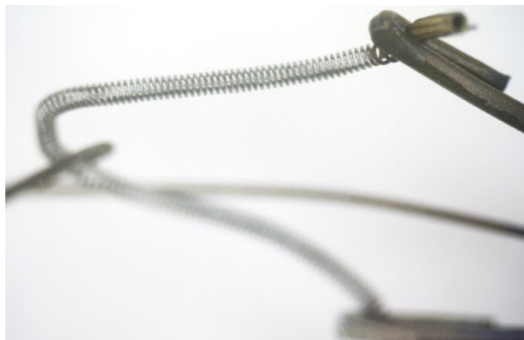
Light Bulb Filament inspected by classic microscope
